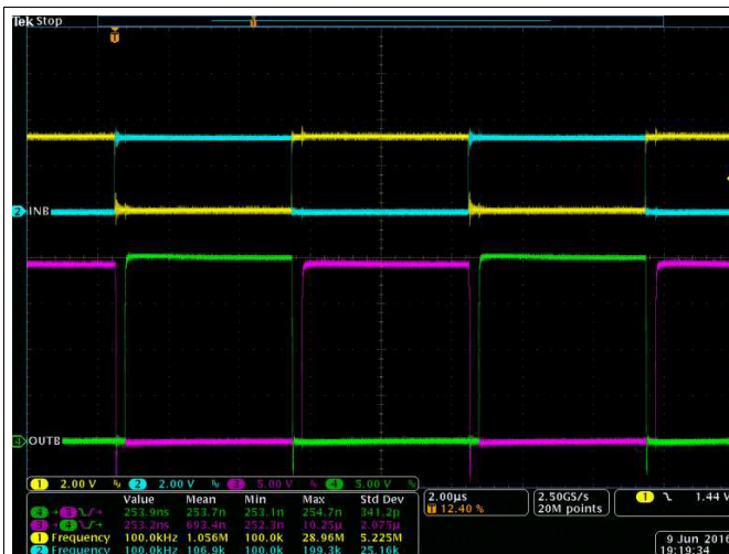
Figure 42. Bench Test Waveform for INA/B and OUTA/B
